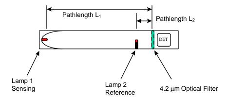
The sensor has two infrared sources (Lamp 1 and Lamp 2), one infrared detector and a narrow band optical filter that passes infrared radiation only at the wavelength absorbed by the gas of interest (4.2 microns for CO<sub>2</sub>). Lamps 1 and 2 are placed in the gas cell at distances L<sub>1</sub> and L<sub>2</sub> respectively from the detector. When a gas concentration C is present in the gas cell, it will absorb the infrared radiation emitted by both the sources according to Beer's Law:
